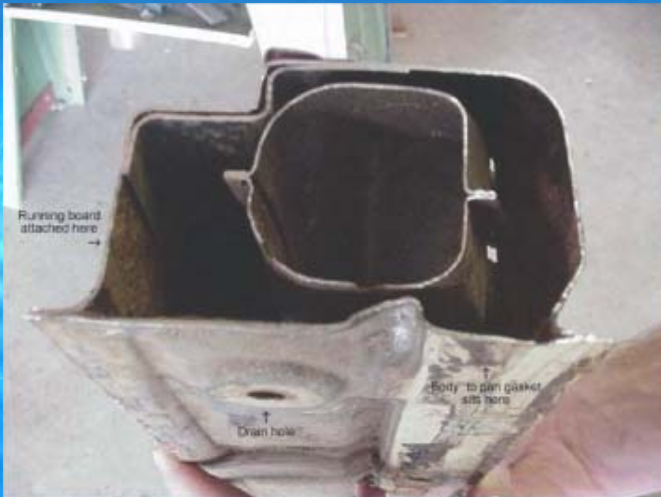
Section through the right hand heater channel. top of page
