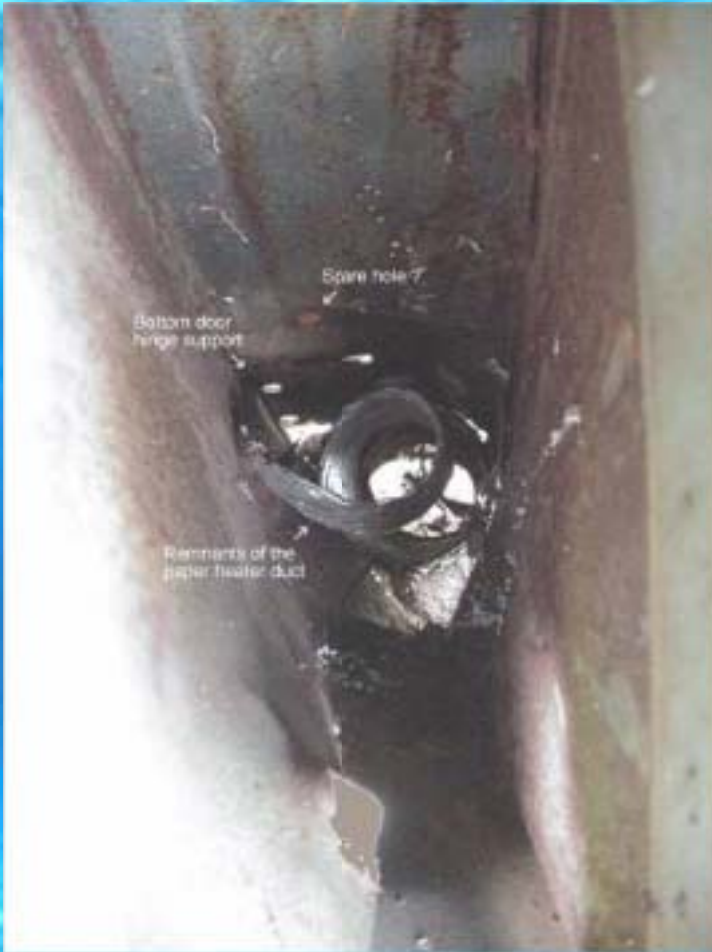
Looking further down into the right hand "A" pillar from the top. top of page
