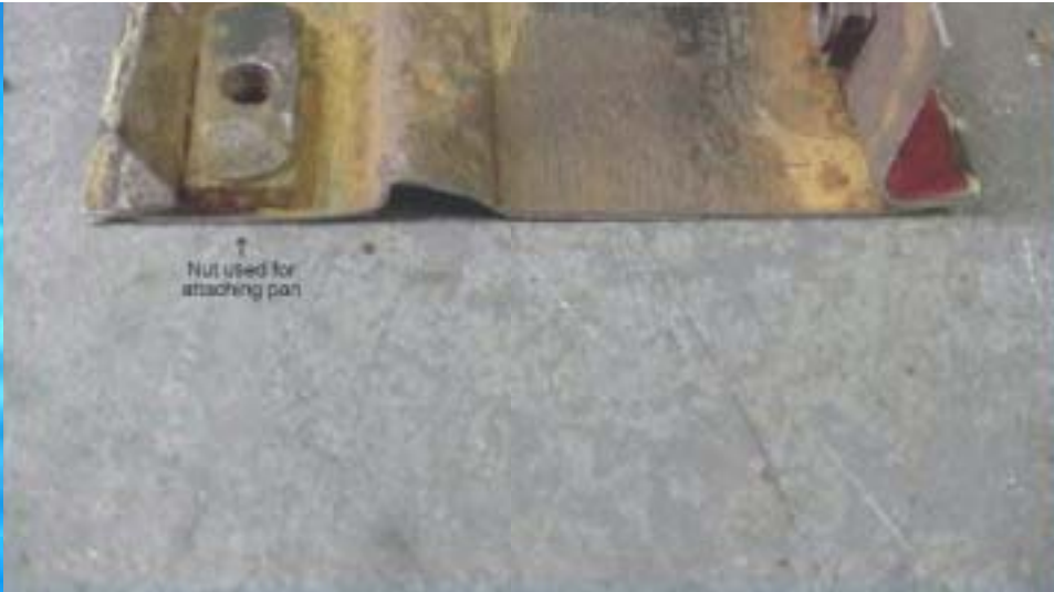
Section through the right hand heater channel the top has also been removed showing the different "nuts" welded to the inside. top of page
